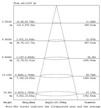
illumination when the luminaire is at different distance.
